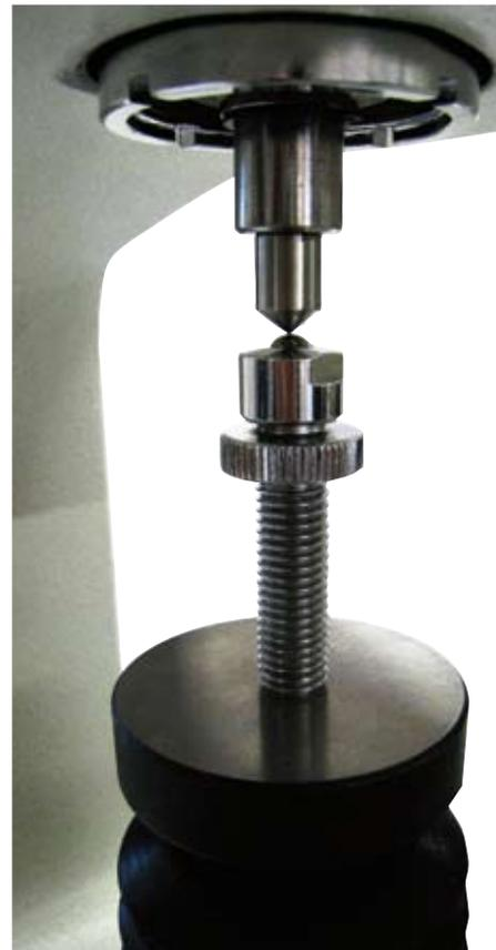
The NR3D hardness tester has a diversified application field. With the different available combinations of standard loads and indenters, it is possible to test very hard materials as well as soft and plastic ones, of different shapes and dimensions.
