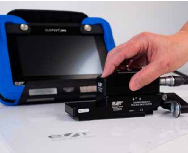
Array sensor with a rotary encoder – for example, for inspecting aircraft skin.
