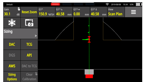
Scan Plan – Lack of fusion or penetration
