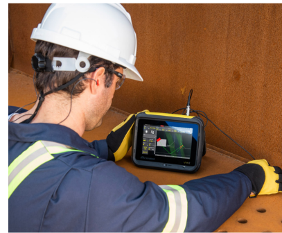
Sonatest WAVE instrument with pre-defined AWS & TKY application setups
