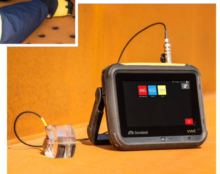
WAVE Interactive Scan-Plan for T-Joint inspection
